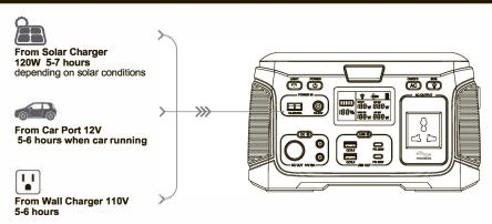
**△ DO NOT CONNECT DEVICE VIA AC OUTPUT PORT WHILE CHARGE THE J500 Mini. RECOMMEND TO DISCONNECT THE J500 Mini WHEN FULL Y CHARGED.**
