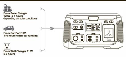
riangle DO NOT CONNECT DEVICE VIA AC OUTPUT PORT WHILE CHARGE THE J300. RECOMMEND TO DISCONNECT THE J300 WHEN FULL Y CHARGED.
