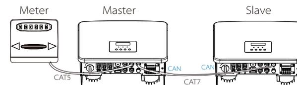
**Step 3:** Disable "settings - Advanced settings-External ATS" on both master inverter and slave inverter.
