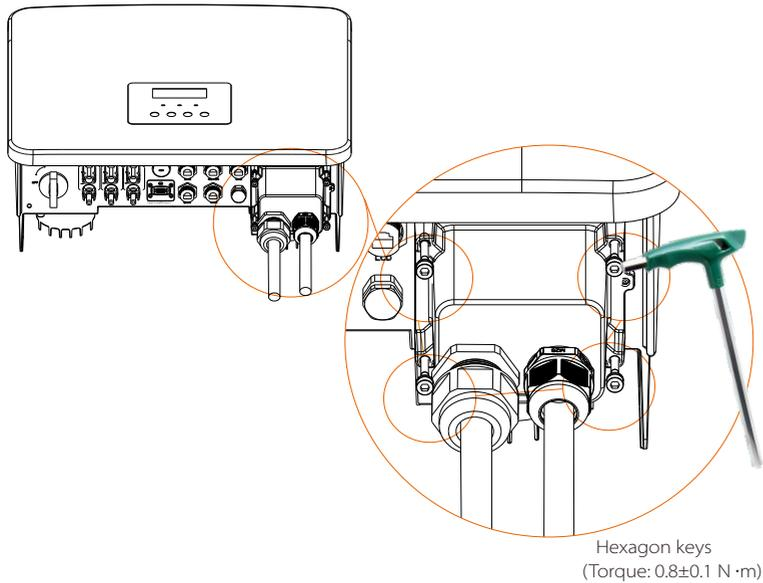
**Step 6.** Tighten the waterproof fastening head.
