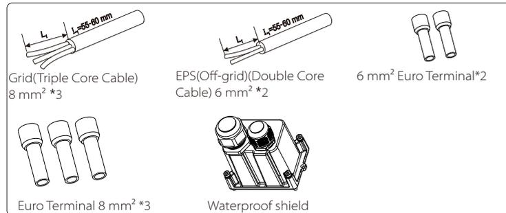
**Step 2:** The Grid and EPS(Off-grid) cables go through the corresponding Grid and EPS(Off-grid) ports of the waterproof shield.
