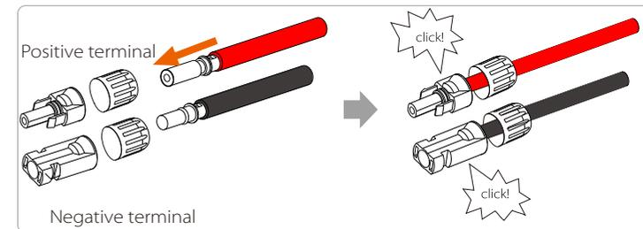
**Step 6.** Tighten the fastening head and insert into the corresponding positive and negative (PV+/PV-) ports of the inverter.
