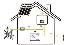
Notice: In the case of grid connection, all working modes work normally when the battery SOC >5%. When the battery charge rate is below 5%, the PV or Grid will first charge the battery SOC 11%, and then return to the working mode selected by the user.
