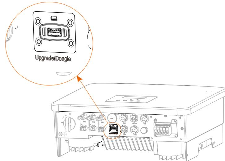
Step 2. Plug WiFi Dongle into the DONGLE port.
