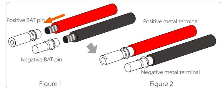
**Step 4.** Tighten the BAT pin contact and the wiring harness to make the connection tight without looseness
