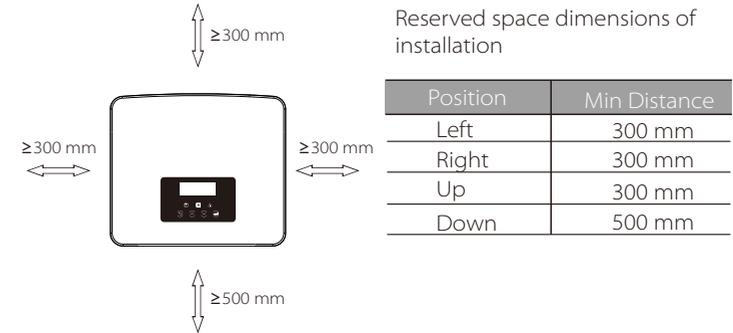
For multi-inverter installation scenarios, the inline installation method is recommended; when the space is insufficient, the recommended method of installation in the form of "products"; it is not recommended to install multiple inverters in stacks. If you choose stack installation, please refer to the installation separation distance below.
