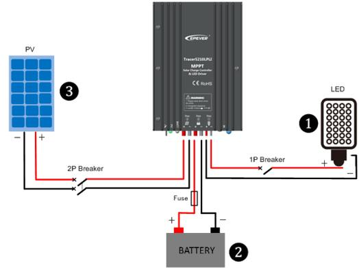
1) Connect components to the charge controller in the sequence as shown above and pay much attention to the “+” and “-”. Please don’t insert the fuse or turn on the breaker during the installation. When disconnecting the system, the order will be reserved.
