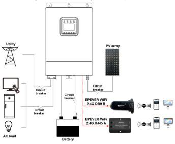
Note: EPEVER WiFi 2.4G RJ45 A is suitable for the controller, inverter, or inverter/charger designed with an RJ45 port. EPEVER WiFi 2.4G DB9 B is ideal for the device designed with a DB9 interface. For detailed connection cables, refer to the connected device's accessories list.
